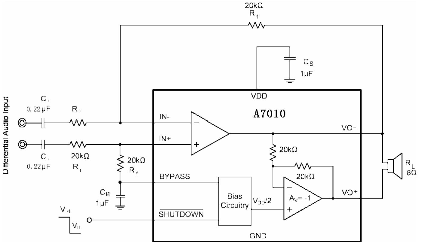
Figure 2. Differential Input application Circuit
